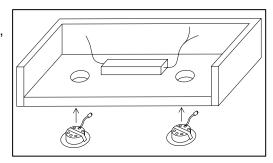
**Installing the electrical components:** The two recessed lamp fittings should be installed into the holes in the mirror canopy.
