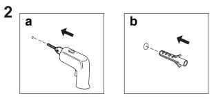
• Using a (Φ6mm) drill make the holes, and insert the wall plugs.
