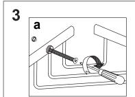
• Thread the screw with the cap washer through the wire basket into the wall plug.
