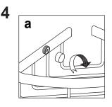
• Once secured affix the cover cap for the screw head .
