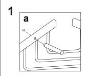
• Determine the position for installation. Put the wire basket in position, make sure it is level, and mark the position for fixing.
